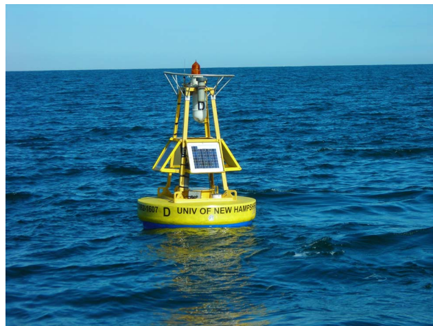
Figure 1. The UNH CO 2 buoy deployed in the coastal Gulf of Maine in North of the Isles of Shoals.
