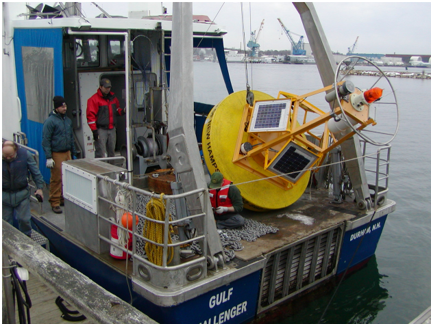
Figure 2. The UNH CO 2 buoy aboard the UNH Research Vessel Gulf Challenger ready to deploy.
