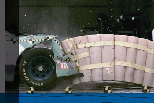
Many common materials, such as rubber or tissue, have nonlinear elastic behavior, where the deformation is not proportional to the applied stress. Battelle has been working with a specific class of materials that have this nonlinear behavior. These hyperelastic materials have properties that vary with the strain rate, or how rapidly the material is deformed.
