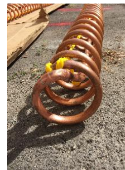
Borehole Heat Exchanger
