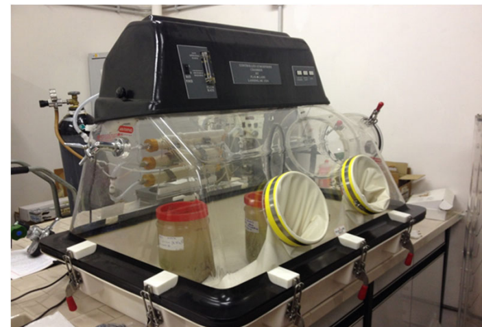
Anaerobic glove box for microcosm preparation.
