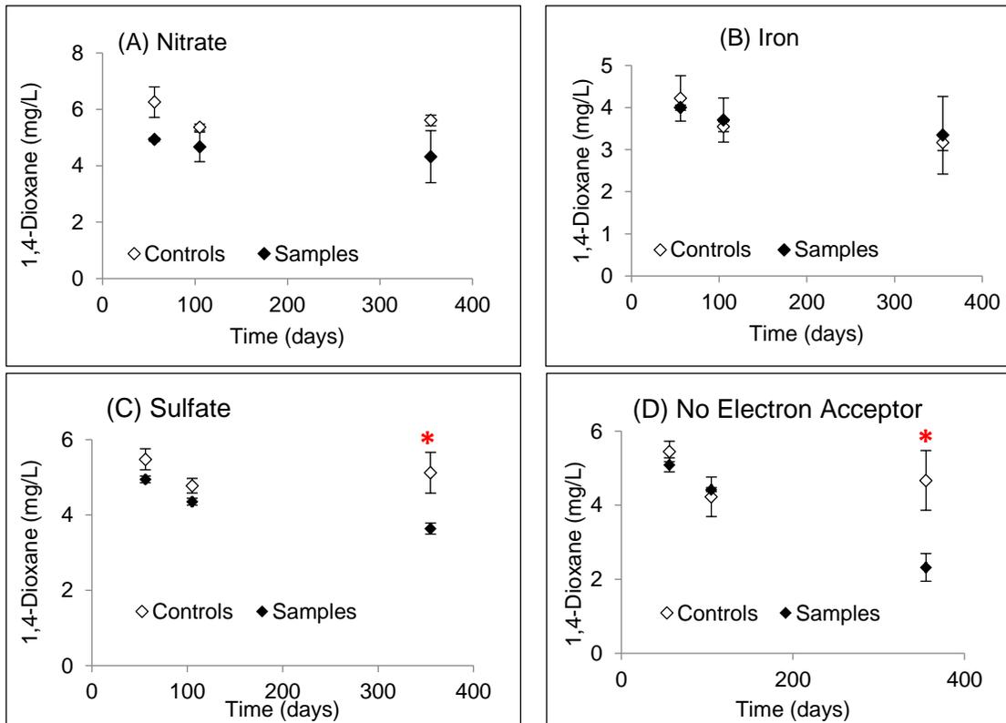
Figure 3. Average 1,4-dioxane concentrations in triplicate microcosms and abiotic controls with inocula from 1,4-dioxane contaminated site 3, amended with nitrate (A), iron (B), sulfate (C) and no amendment (D). The bars represent the standard deviation and the red asterisk indicate significant differences between samples and controls.
