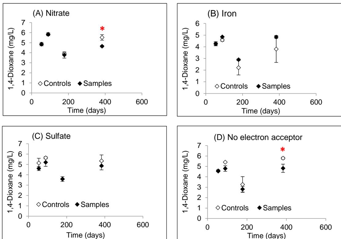
**Figure 4.** Average 1,4-dioxane concentrations in triplicate microcosms and abiotic controls with inocula from 1,4-dioxane contaminated site 1, amended with nitrate (A), iron (B), sulfate (C) and no amendment (D). The bars represent the standard deviation and the red asterisk indicate significant differences between samples and controls
