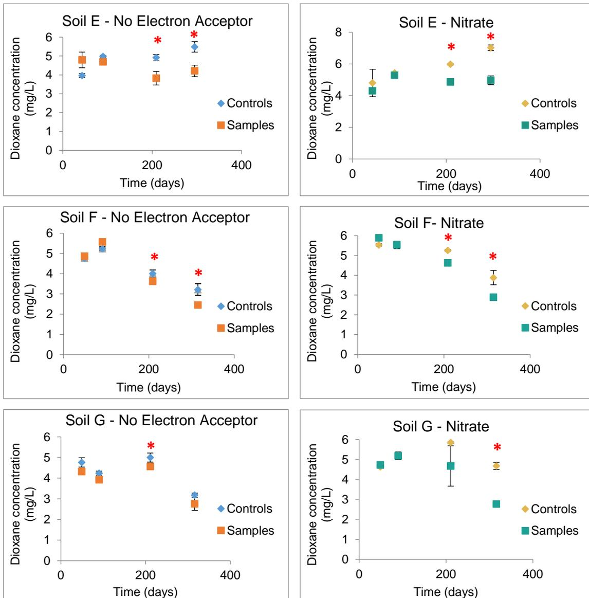
**Figure 1. Average 1,4-dioxane concentrations in triplicate microcosms and abiotic controls with inocula from agricultural soils, with no amendment (left) and amended with nitrate (right). The bars represent the standard deviation and the red asterisk indicate significant differences between samples and controls ( $p < 0.05$ ).**
