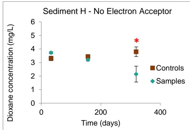
Figure 2. Average 1,4-dioxane concentrations in triplicate microcosms and abiotic controls with inocula from river sediments with no amendment. The bars represent the standard deviation and the red asterisk indicate significant differences between samples and controls.
