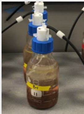
Triplicate bottles for anaerobic treatments
