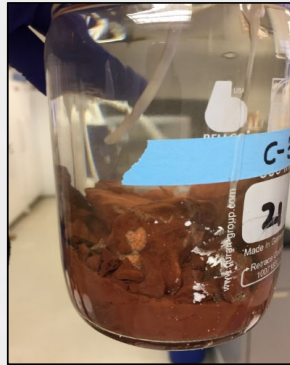
Combined all triplicate bottles into one to reach DO saturation
