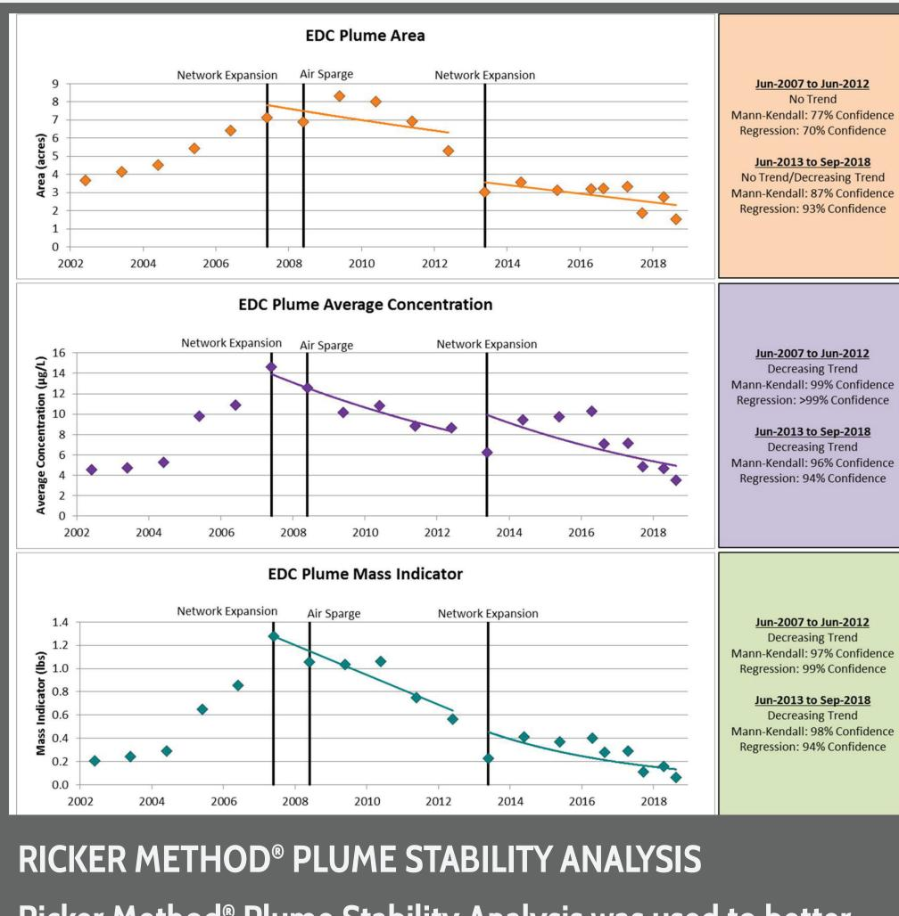
Ricker Method<sup>®</sup> Plume Stability Analysis was used to better assess the effectiveness of the onsite remediation systems with a focus on the groundwater extraction system.
