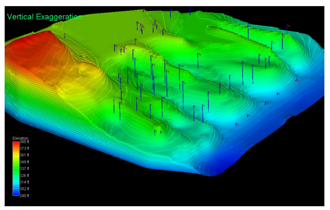
Step 2 - Bedrock surface elevations entered into the EVS system to generate model
