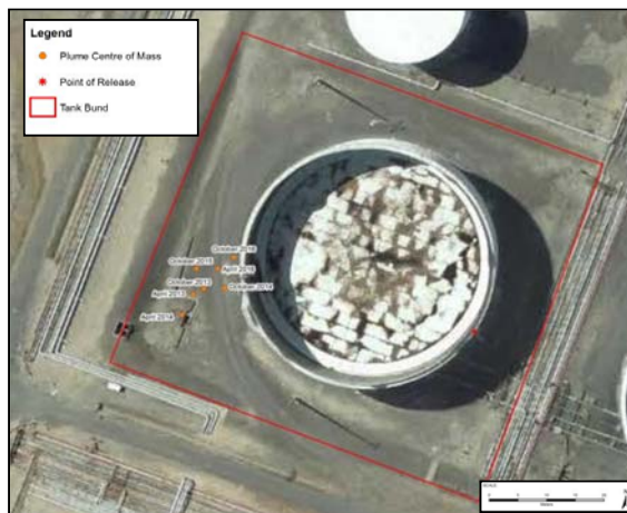
FIGURE 7. Plume center of mass movement from 2013 to 2016.
