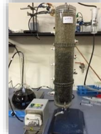
Clay-Coarse Sand Column
