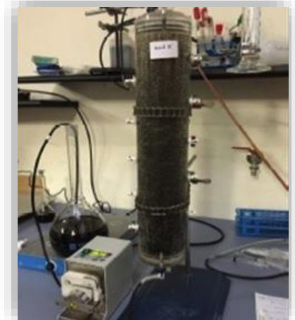
Clay-Coarse Sand Column
