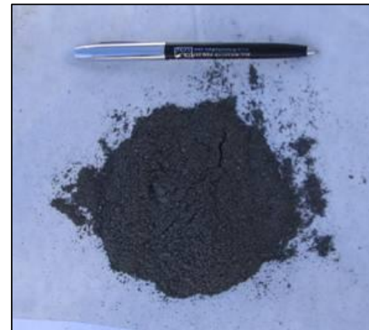
Granular EHC powder – composed of microZVI and solid plant fibers
