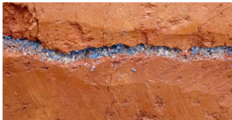
Sand seam emplaced via hydraulic fracturing (courtesy of FRx)
