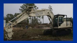
Modified Lang Working Depth: 22 feet (with extension) Constant Power: 200 HP Dual Motors: No Automatic Power Control: No Reach Depth in Clay: Sometimes Blend Weathered Rock: Maybe
