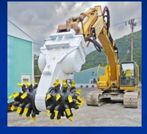
Redox Tech Custom Working Depth: 22 feet Constant Power: 295 HP Dual Motors: Yes Automatic Power Control: Yes Reach Working Depth in Clay: Yes Blend Weathered Rock: Yes
