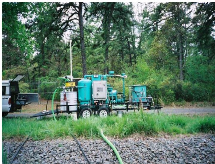
FIGURE 3. DPE system during pilot study.
