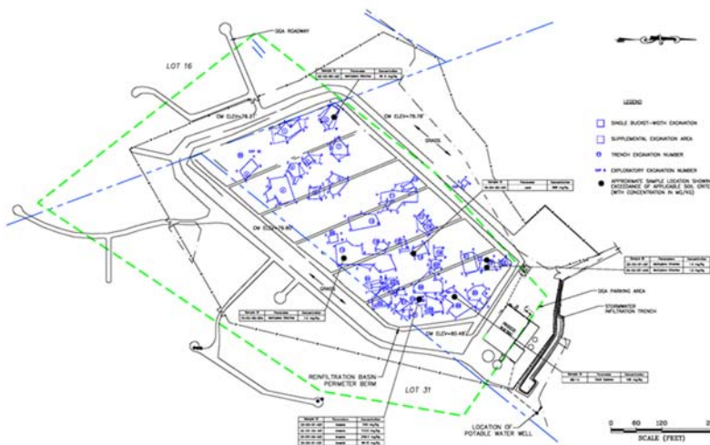
FIGURE 1. Site plan showing soil excavation areas and sample locations exceeding applicable soil criteria.
