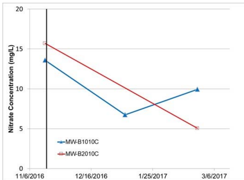
FIGURE 8. Nitrate concentration in two wells approximately 3 meters downgradient of PRB.
