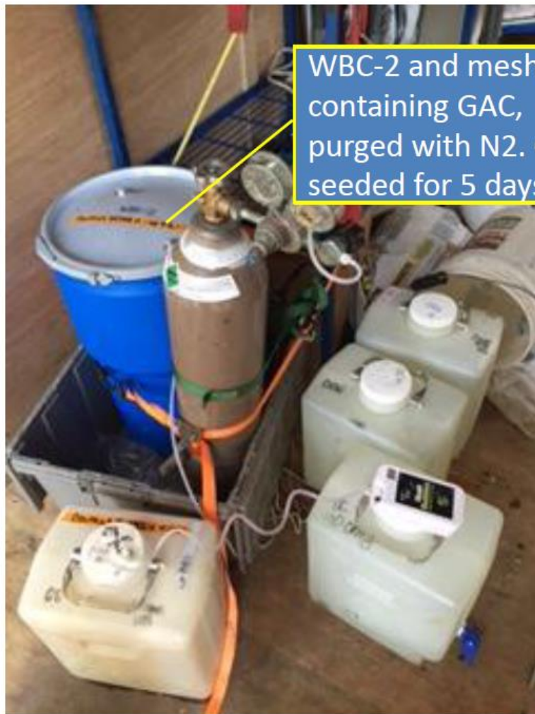
Bacteria transported to site in trailer along with a nitrogen tank for WBC-2.
