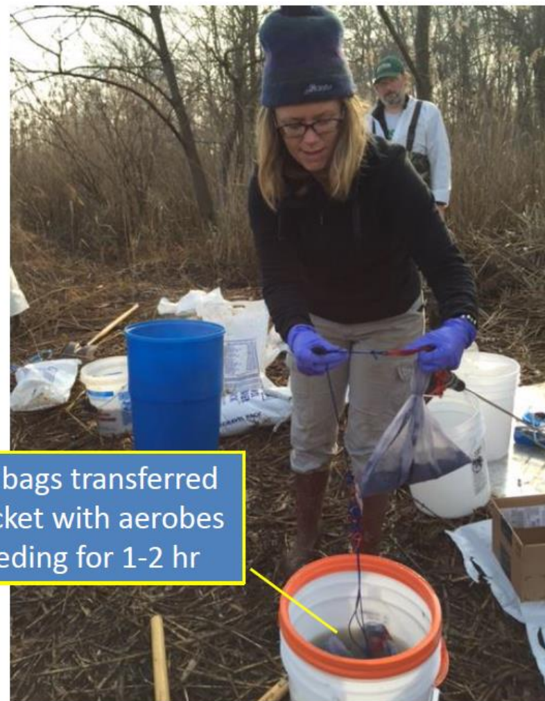
WBC-2 seeded GAC in mesh bags transferred for seeding with 15B aerobes
