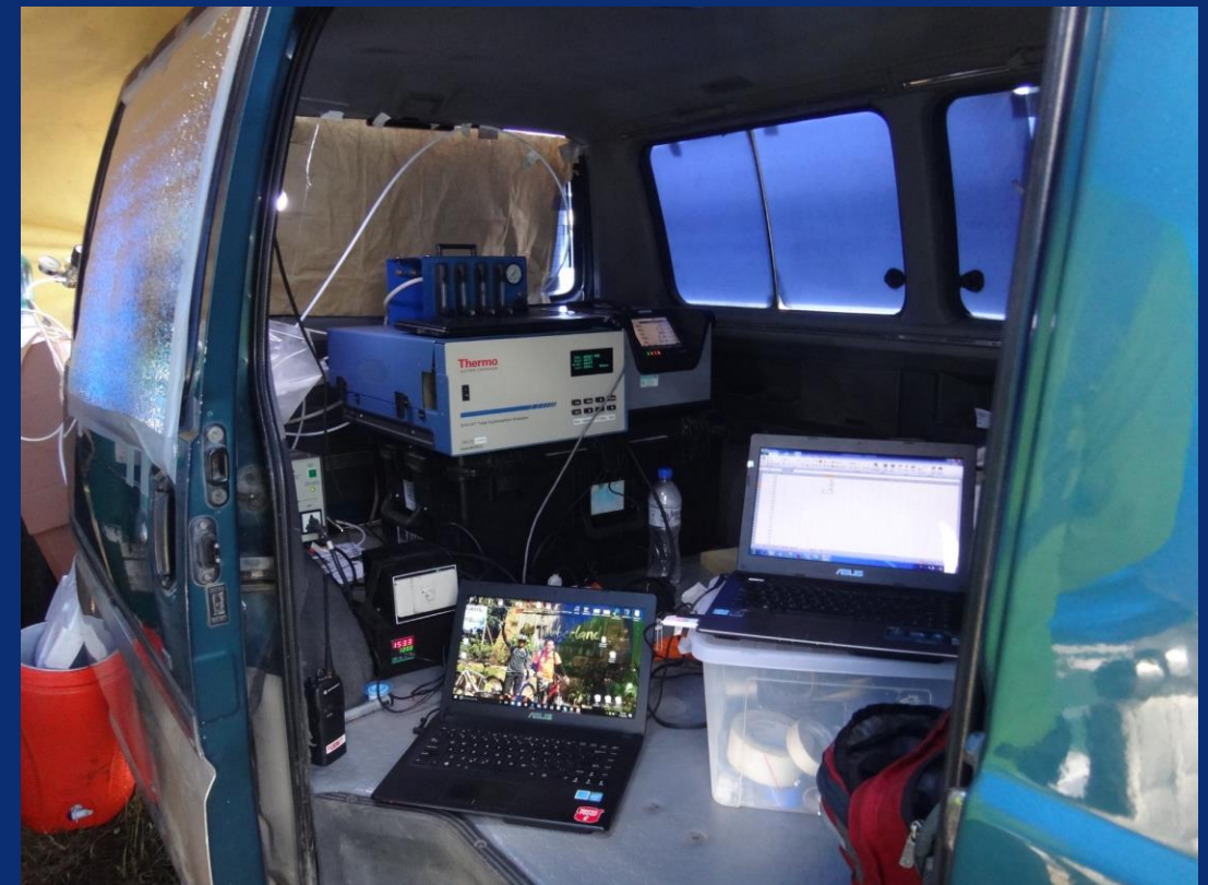
Combustion Gas Monitoring System
