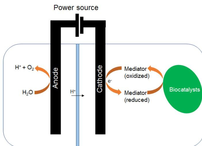
**FIGURE 4. Electron transfer from electrode to biocatalysts through use of mediators in the microbial electrosynthesis cell.**
