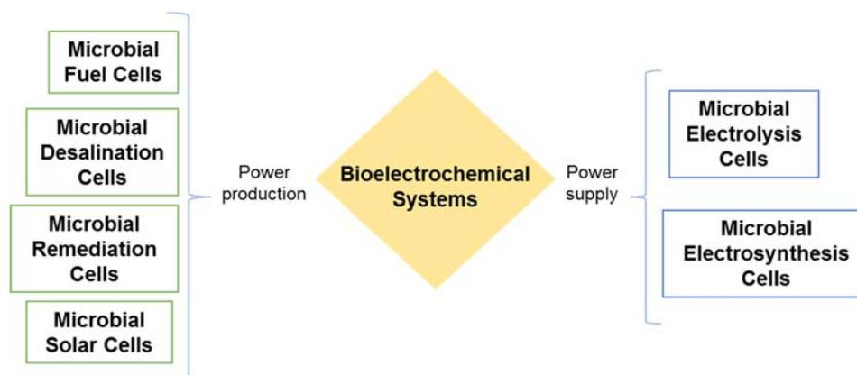
**FIGURE 1. Types of bioelectrochemical systems.**
