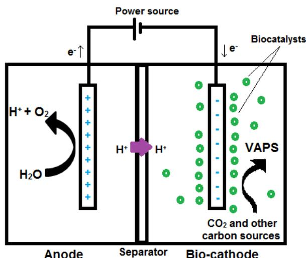
FIGURE 3. A typical two-chamber microbial electrosynthesis cell.
