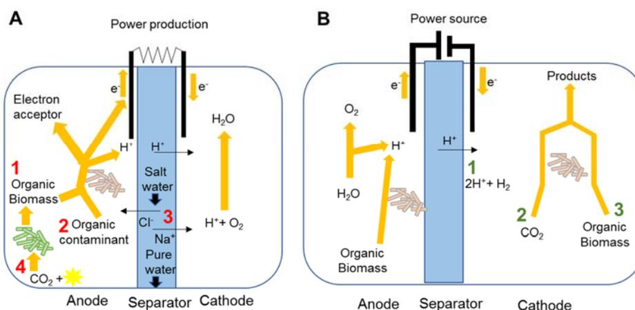
**FIGURE 2. (A) Bioelectrochemical systems with power production. Red numbers inside anodic chamber of the figure indicate BES type: 1, Microbial Fuel Cells; 2, Microbial Remediation Cells, 3, Microbial Desalination Cells; 4, Microbial Solar Cells;**
