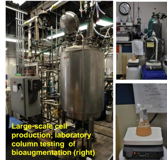
Large-scale cell production; laboratory column testing of bioaugmentation (right)
