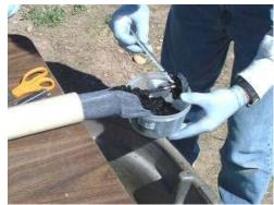
1. Contaminant adsorbed onto passive flux meter over time to get Concentration
