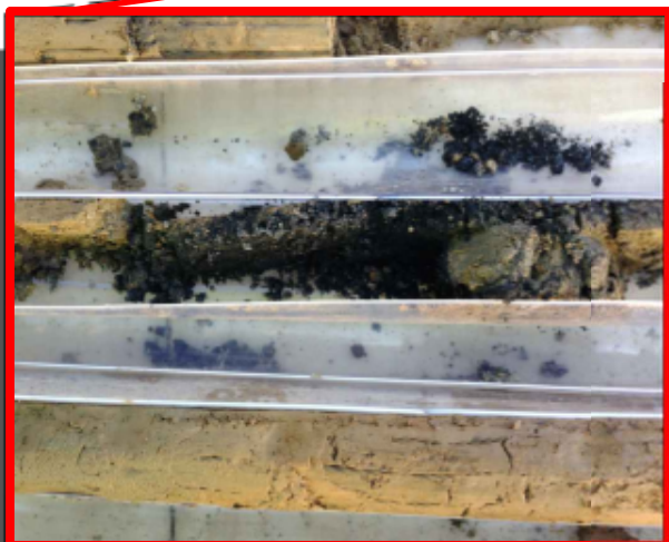
Soil Core Close Up From Boring SB186
