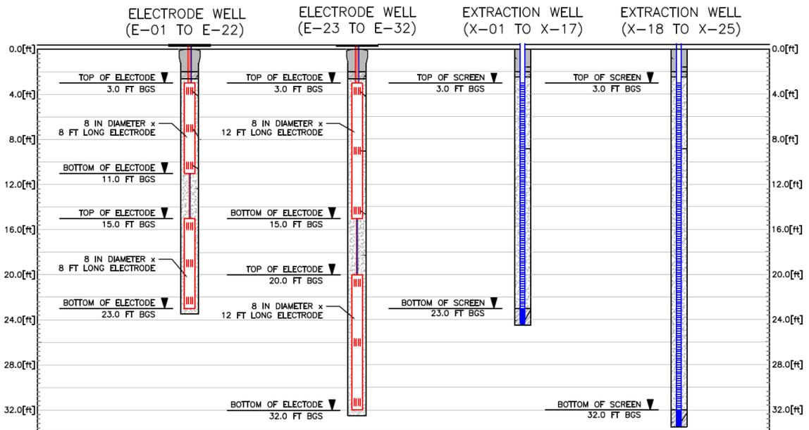
FIGURE 2. Electrode and extraction well construction details within the pseudo symmetry element.
