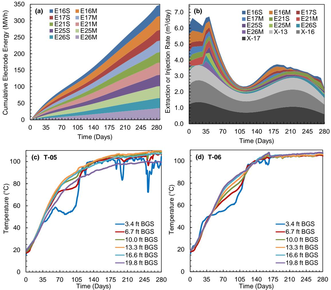
**FIGURE 3. Field measurements of (a) cumulative electrode energy, (b) water extraction or injection rate, (c) temperature at T-05, and (d) temperature at T-06.**
