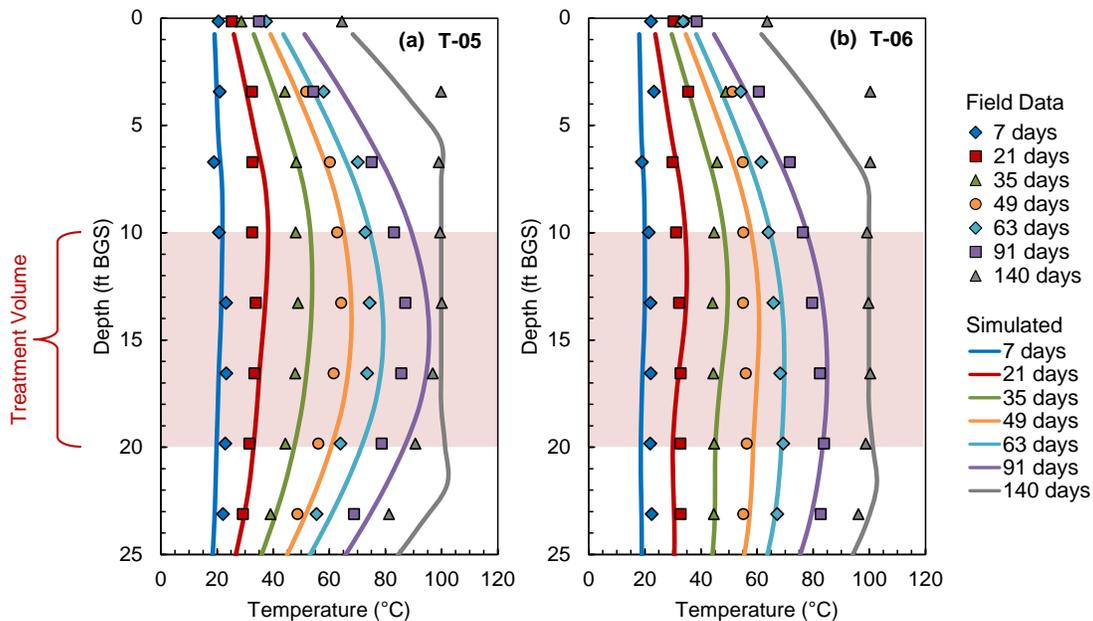
**FIGURE 4. Comparison of the simulated and measured responses at temperature monitoring points (a) T-05 and (b) T-06.**
