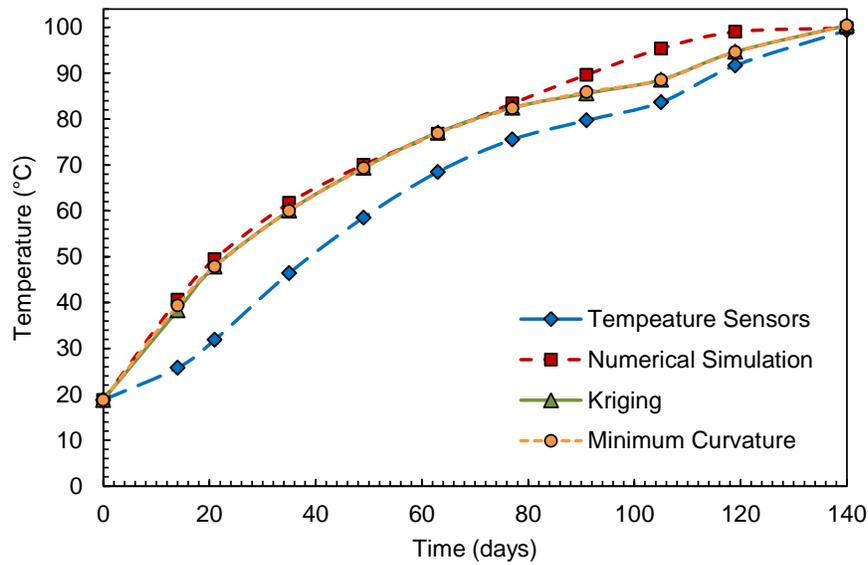
**FIGURE 8. Average temperatures (i) measured in the field at sensors T-05 and T-06 and (ii) calculated in the 10 ft BGS slice using the various contouring methods.**
