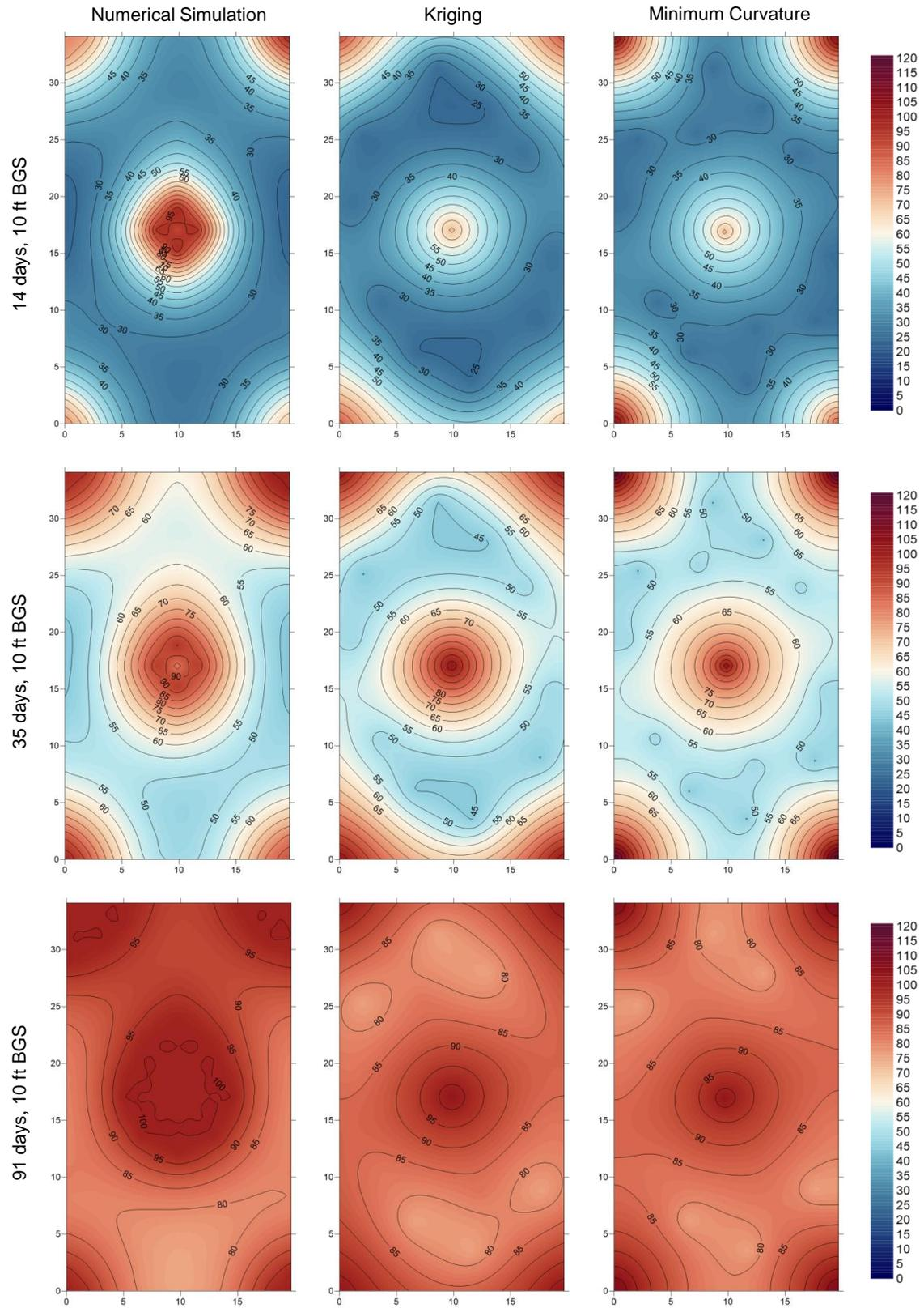
**FIGURE 7. Comparison of history matched numerical simulations to thermal contours generated by contouring with Kriging and Minimum Curvature.**
