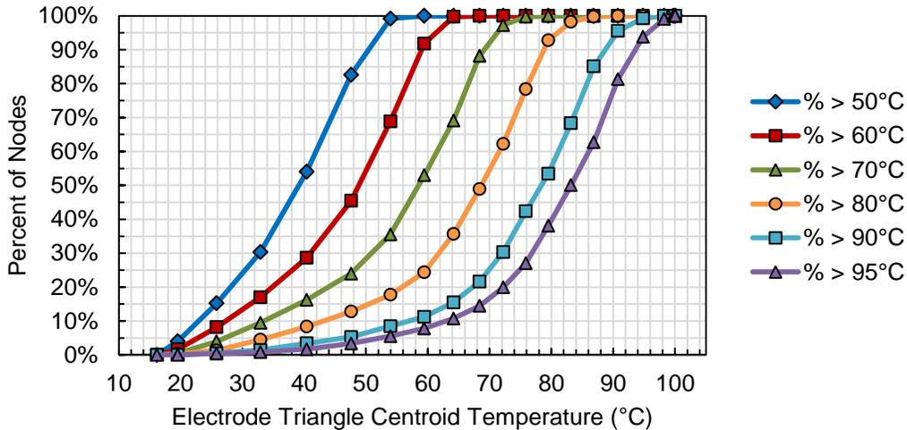
**FIGURE 6. Percent of simulated treatment volume that has achieved a temperature target, given the average temperature at the centroid of the triangle formed by electrodes E-21, E-25, and E-26.**
