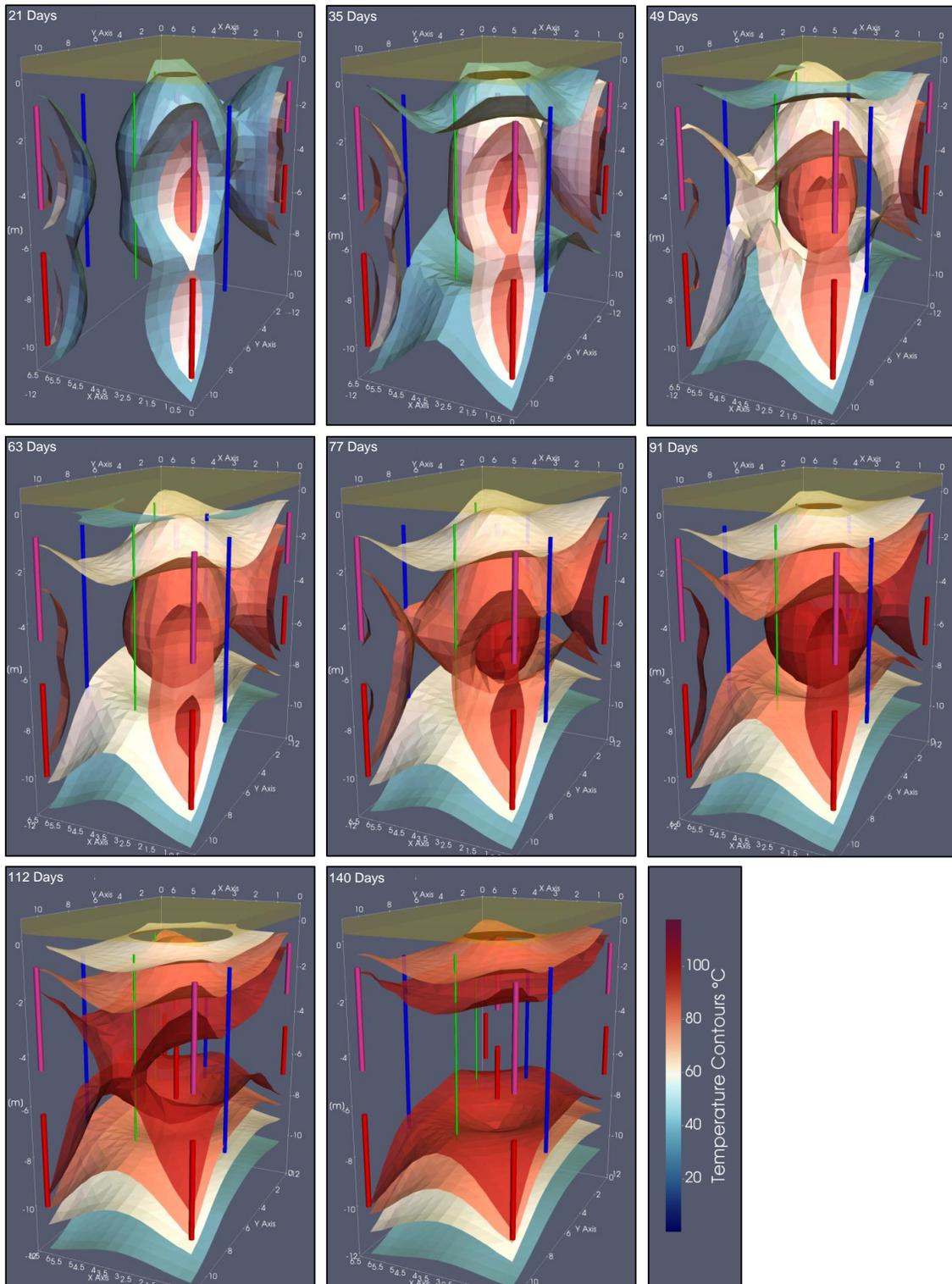
**FIGURE 5. Simulated three dimensional temperature distributions for the pseudo symmetry element with 40, 60, 80, and 100°C isotherms contoured.**
