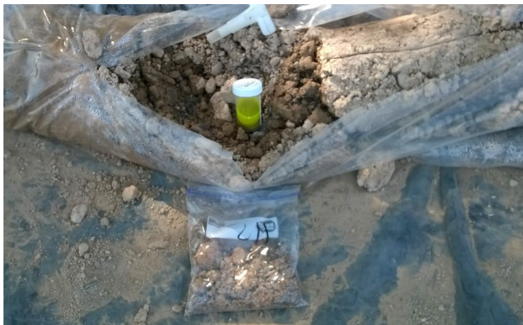
Dye tests have been successfully used to observe waste oil NAPL and jet fuel in soils.
