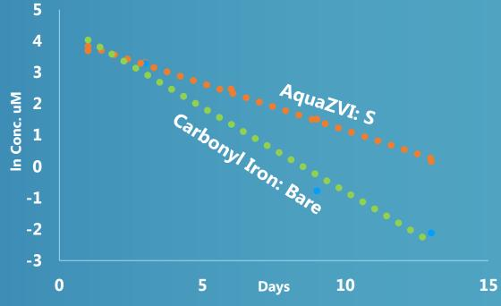
Bare iron degrades 1,1,1-TCA faster than sulfidated iron – opposite result of TCE
