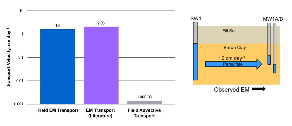
$J_{EM} = U_i C_i i_e$  Effective Ionic Mobility (U<sub>i</sub>), Concentration (C<sub>i</sub>), Voltage Gradient (i<sub>e</sub>)
