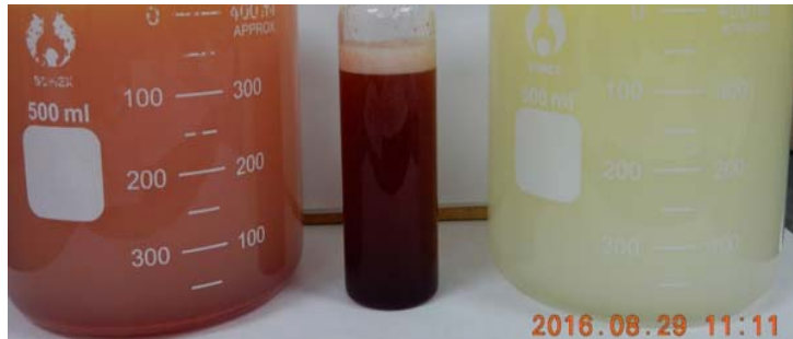
Photograph 1. Provect-ERD CH4™ 15:1 Water:Oil (Left), 85% Carbon + 4% AMR Self-Emulsifiable Oil Concentrate (Middle), and 85% Carbon Self-Emulsifiable Oil Concentrate , no AMR (Right).
