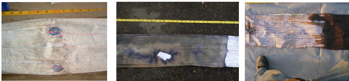
Figure 1. Examples of DNAPL stains on the NAPL cover interior. Left to right: TCE, TCE with oil, and coal tar
