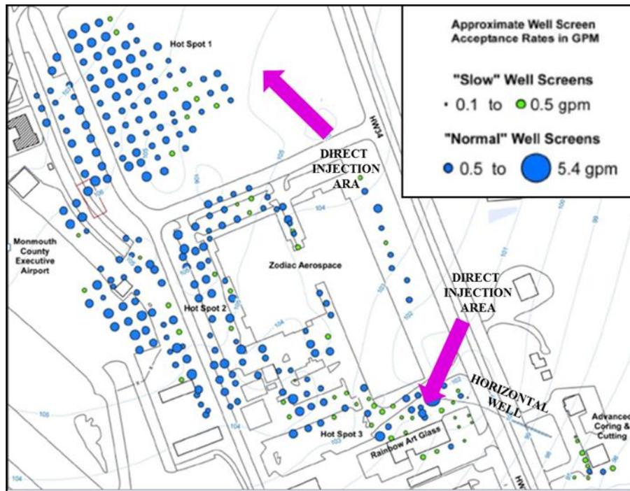
**FIGURE 5. Injection well screen amendment acceptance rates across the site**
