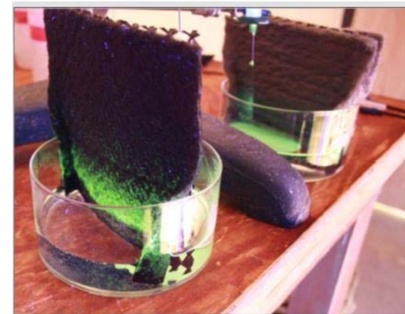
Polymer geocomposite wicking hydrocarbons
