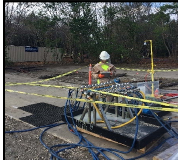
One of two 16-leg injection manifolds
