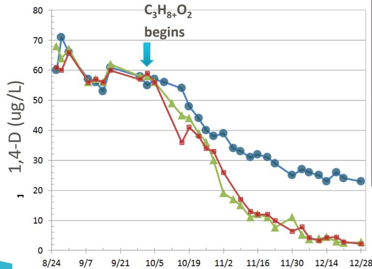
GW recirculation with propane and oxygen injection to create an underground ACB bio-reactor.
