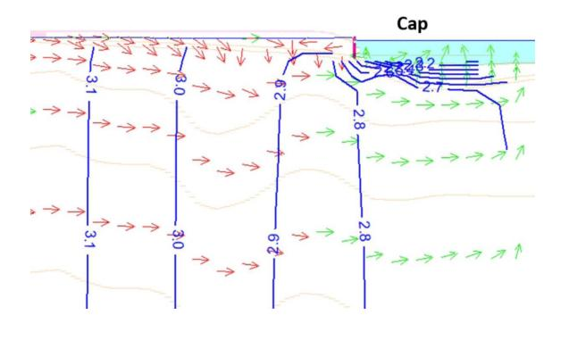
Predicted Groundwater Flow **Under Capped Condition**
