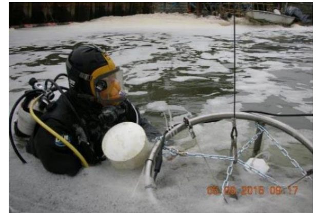
Seepage Meter Installation
