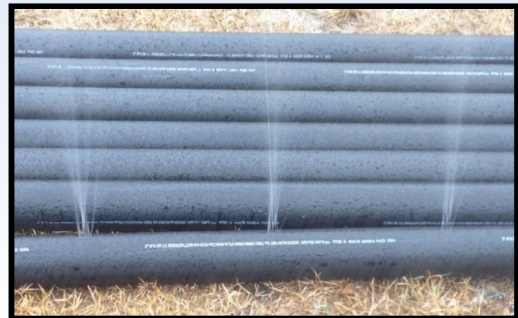
Water being pumped through horizontal remediation well to demonstrate uniform flow through well screen
