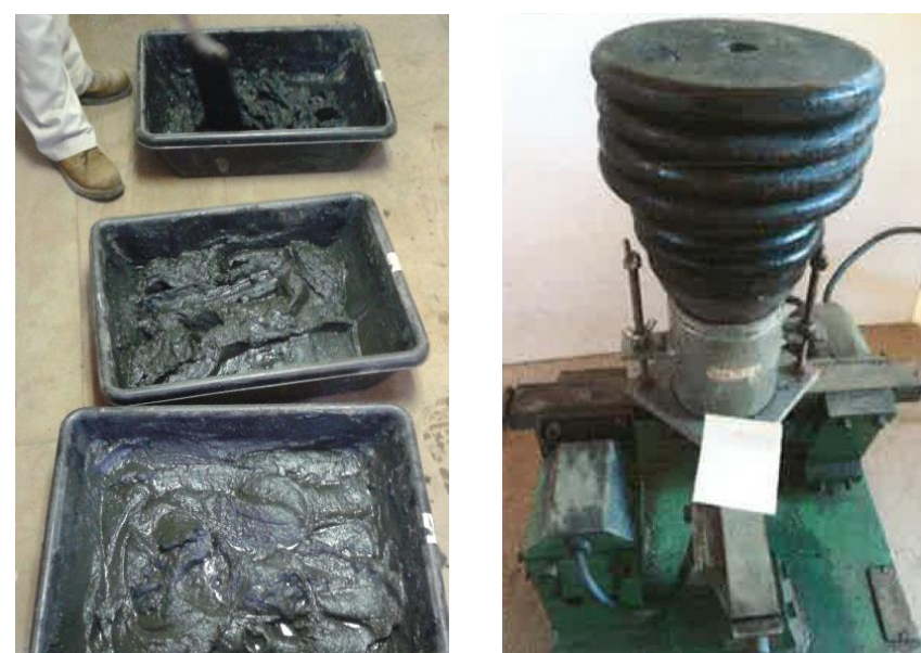
FIGURE 4: Homogenized material (left) and vibratory table for liquid release testing (right).
