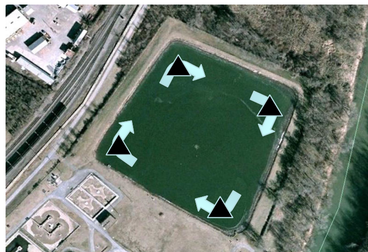
Approach II - Mix Bioamended SediMite with circulation pumps
