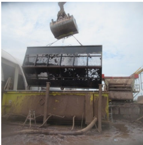
Dewatering Basket to separate "oatmeal"
