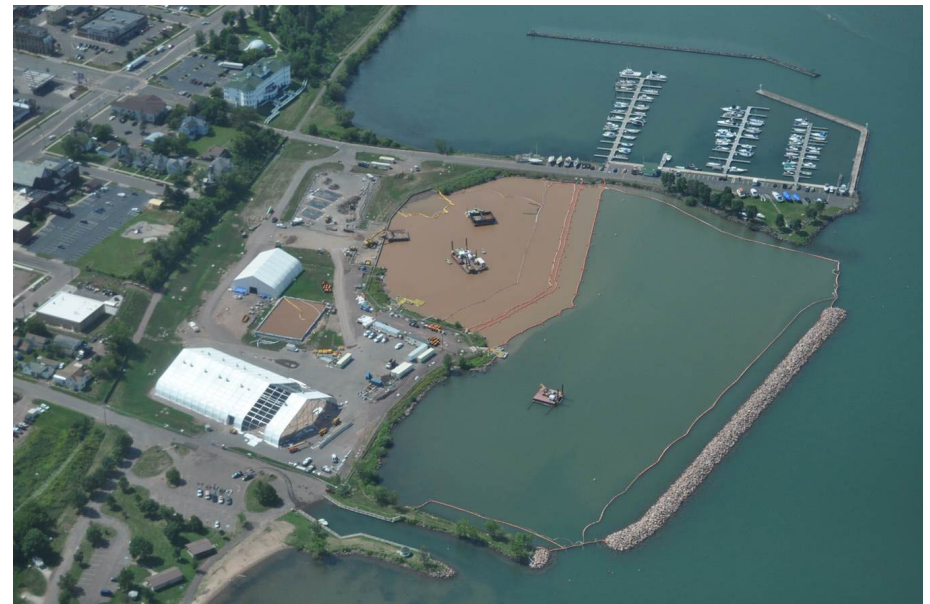
Mechanical Dredging within Barrier Curtain System
