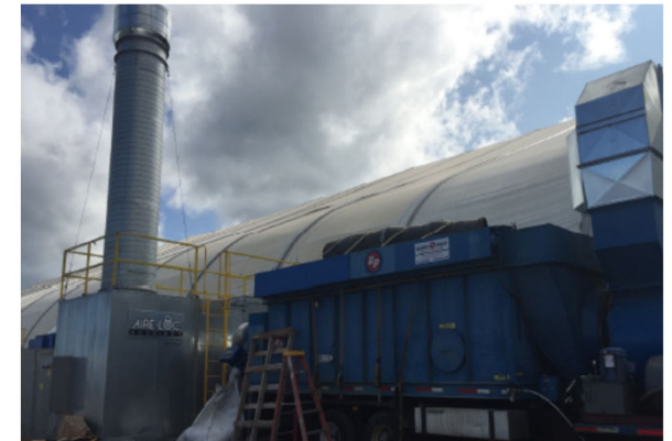
Dust Collectors – reduce lime dust in tent atmosphere
