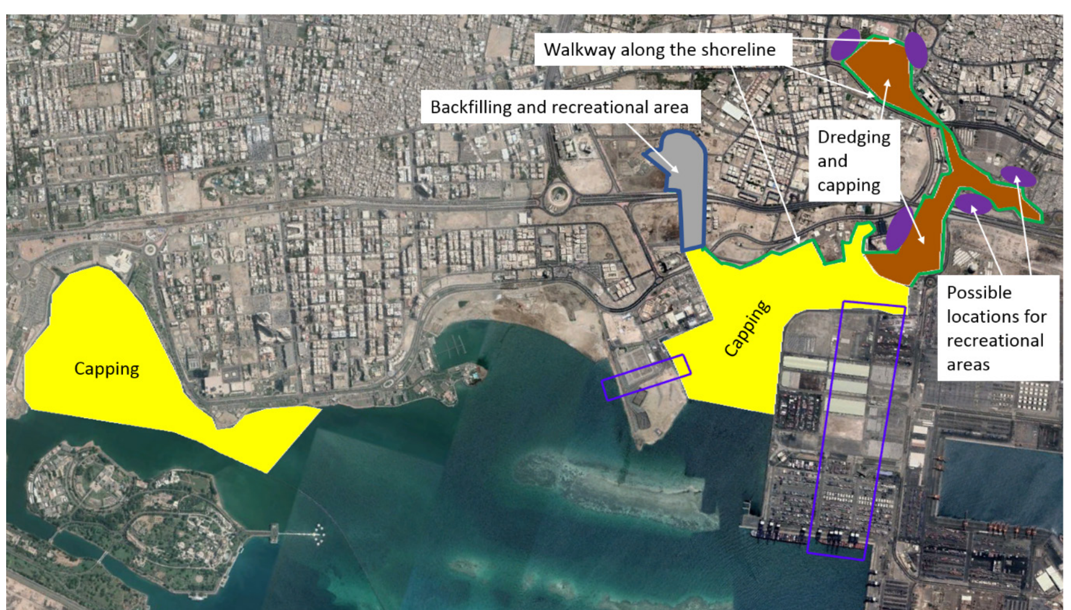
Figure 7. Illustration of the different remediation measures implemented in design 1.
