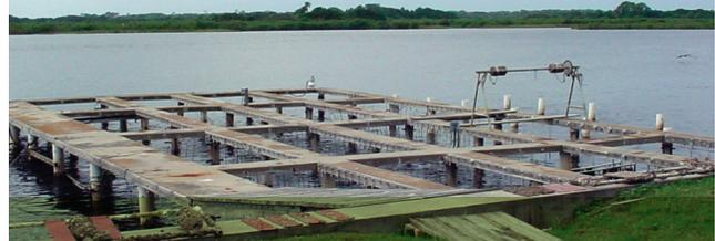
Marine Immersion Dock for antifouling, fouling release, and splash-zone tests
