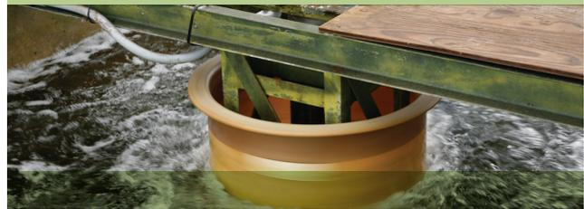
"Paint Wheel" rotating at 16 knots during dynamic test of hull coatings for ASTM D4939 "Subjecting Marine Antifouling Coating to Biofouling and Fluid Shear Forces in Natural Seawater"
