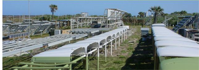
Outdoor Testing of Automotive Components at Battelle's Marine Atmospheric Site
