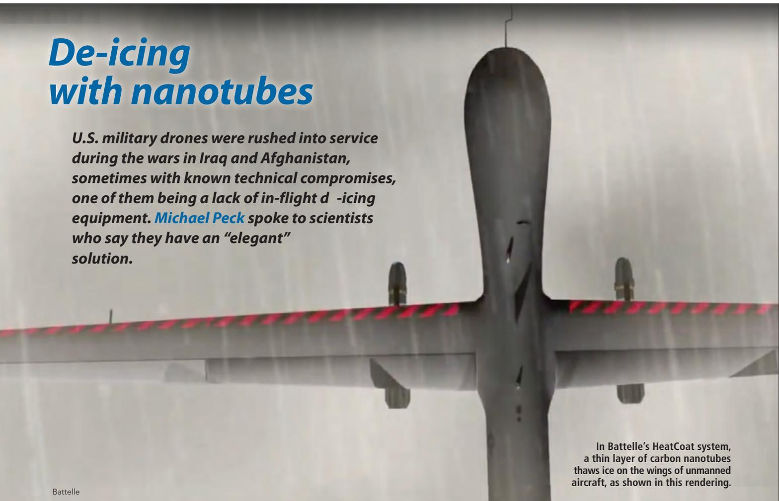
In Battelle's HeatCoat system, a thin layer of carbon nanotubes thaws ice on the wings of unmanned aircraft, as shown in this rendering.
