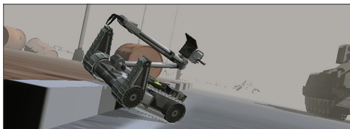
MTRS MK1/PackBot simulation in Battelle's EOD Robot Training Simulator (ERTS).
