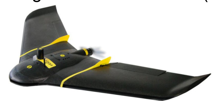
Figure 4. Unmanned aerial system- SenseFly eBee+
