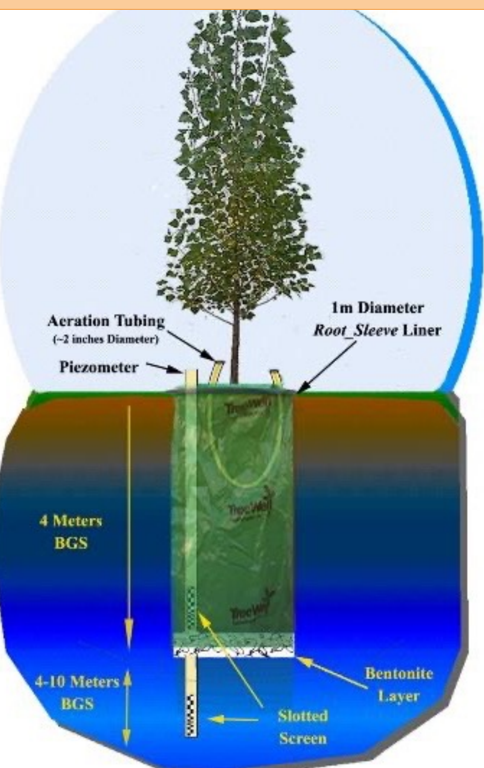
Schematic of Straw TreeWell Unit
