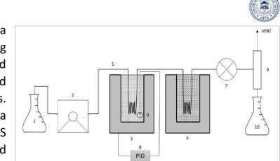
Figure 3. Process flow diagram of the continuous HALT reacto used in the destruction of PFAS in AFFF-impacted wate (Technology HA-1) (Pinkard et al., 2023).
