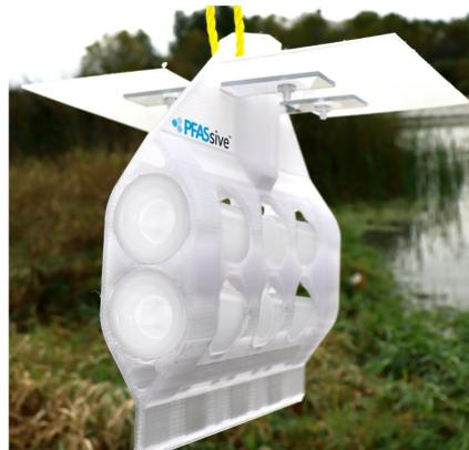
**FIGURE 1:** PFAS Passive Sampler in 3D Printed Frame
