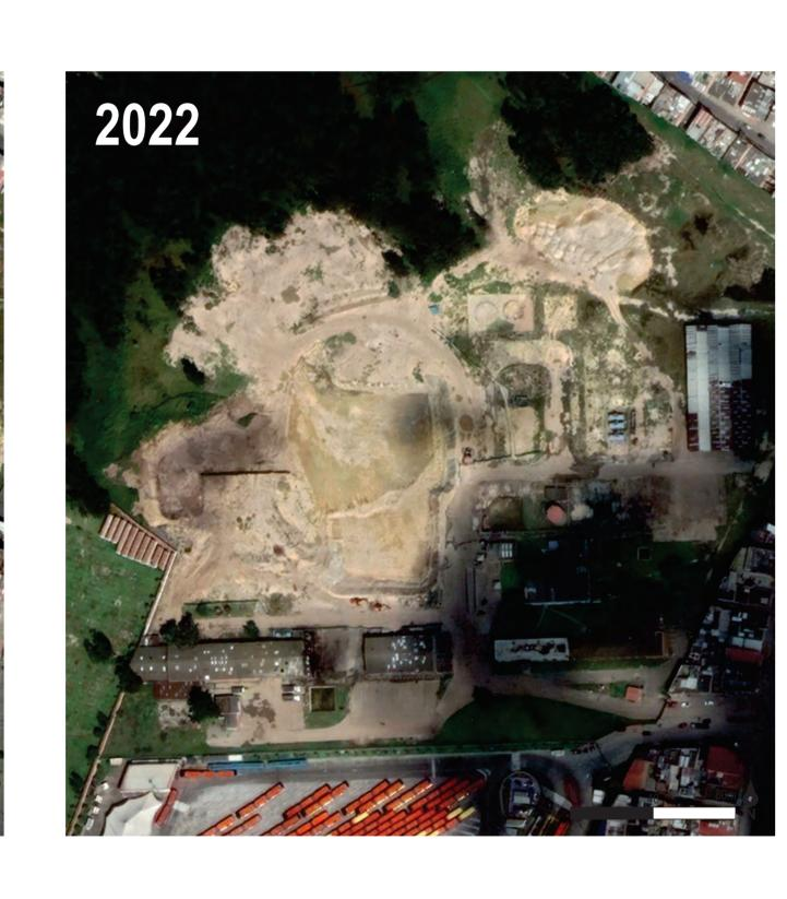
Initially the company conducted a poor site investigation and the identified LNAPL from the area was subjected to a huge excavation removing more than 100,000 metric tons in one year. Considering the excavation was still revealing more and more free phase occurrences, it was decided to identify a company with the necessary expertise to carry out a new investigation to understand the hydrogeological conceptual model and the contamination of the area.
