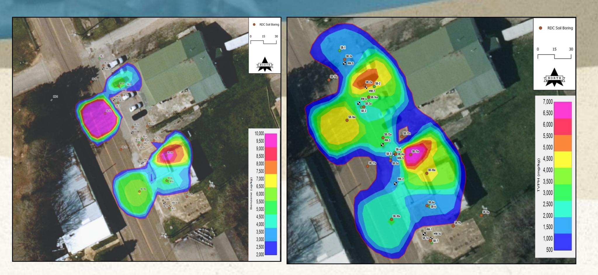
• Reduce LNAPL mobility in short term by establishing an in situ platform for carbon adsorption Enhance long-term reduction of VOCs and total volatile petroleum hydrocarbon (TVPH) mass utilizing BOS 200<sup>®</sup> and BOS 200+<sup>®</sup> biological processes
