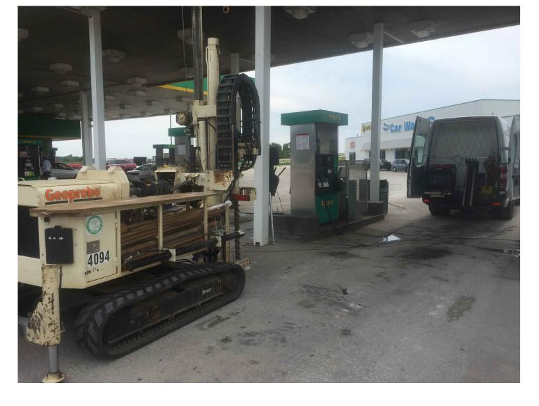
The technology includes a probe which houses a fiber optic cable that transmits light through a sapphire window in the side of the probe, exposing the soil to UV light. The UV light stimulates the emission of photons from polycyclic aromatic hydrocarbons (PAHs) present in petroleum hydrocarbons. The emitted waveform is then divided into four wavelengths which roughly correspond to product types.
