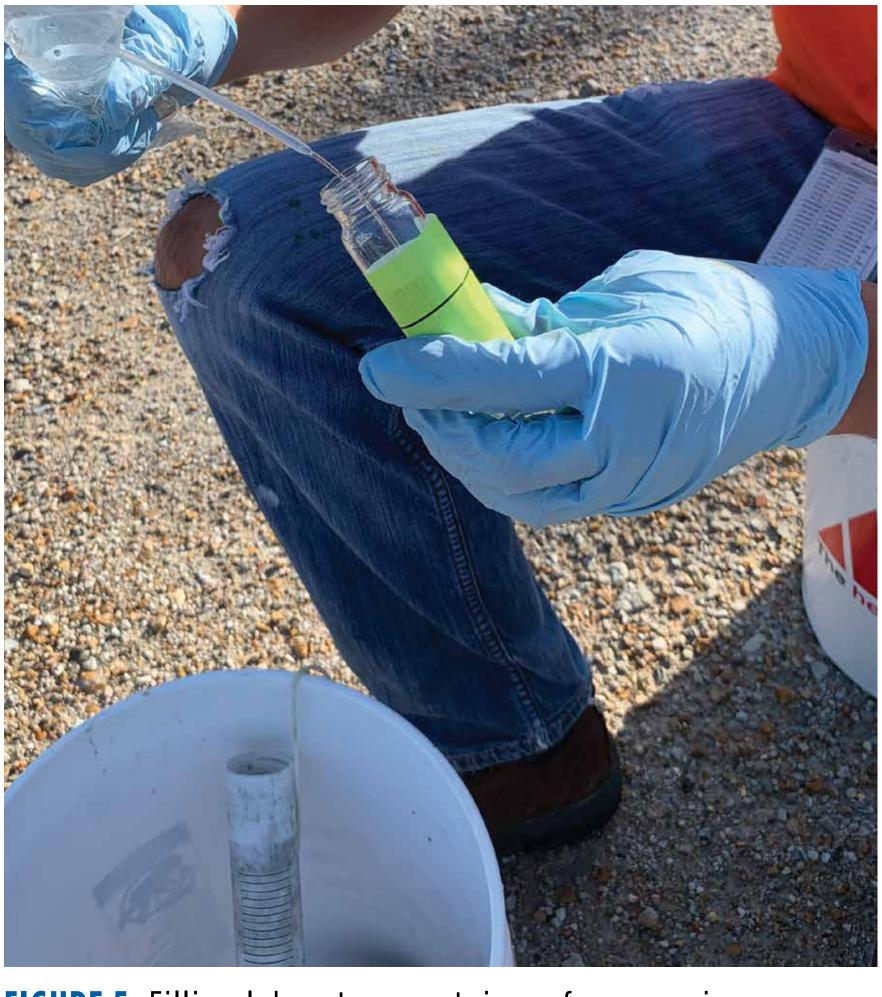
**FIGURE 5**: Filling laboratory containers from passive sampling bags deployed in the monitoring well.
