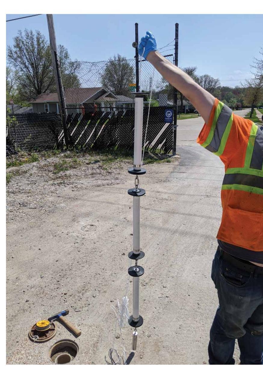
**FIGURE 2**: In situ microcosm assembly: MNA unit (top), BioStim unit (middle), bioaugmentation unit (bottom).
