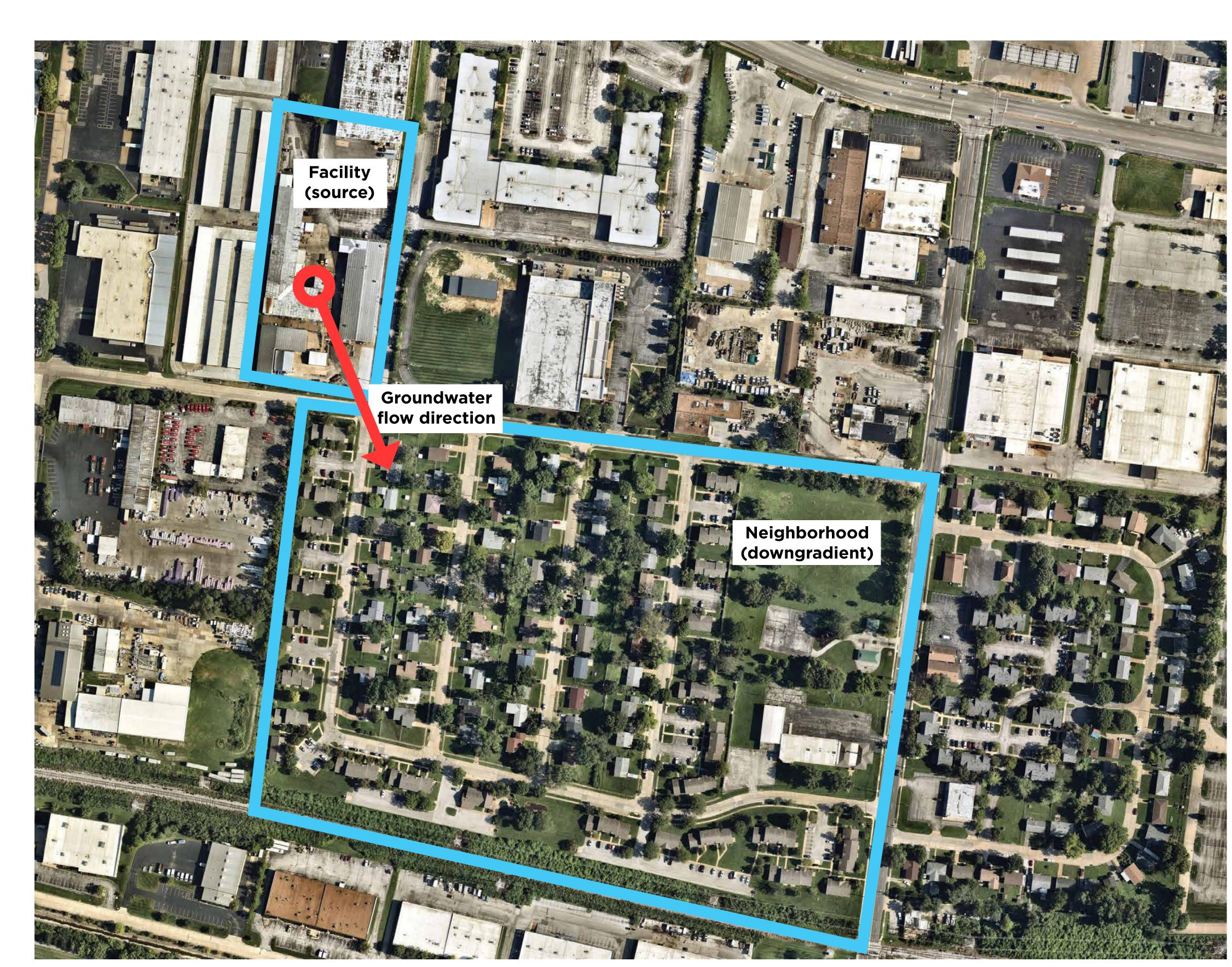
**FIGURE 1**: Aerial image of the facility and downgradient residential neighborhood. The condensed nature of the residential buildings provided unique challenges associated with equipment access for subsurface characterization activities.
