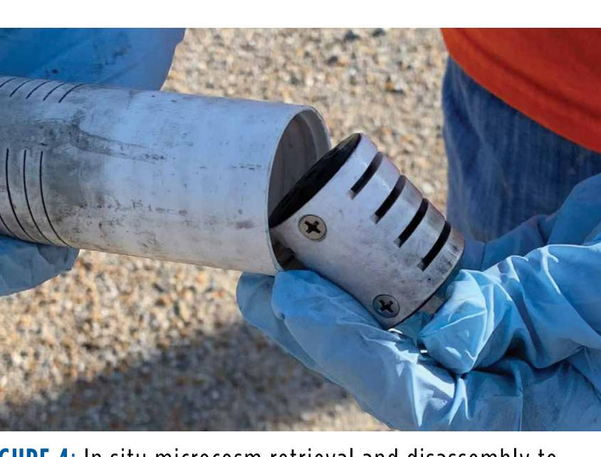
**FIGURE 4**: In situ microcosm retrieval and disassembly to obtain samples for laboratory analysis.
