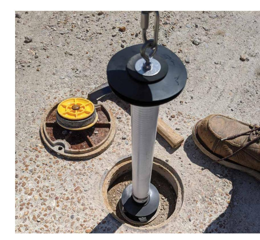
FIGURE 3: In situ microcosm assembly being lowered into monitoring well.
