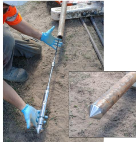
Drivepoint FO assembly; knockout tip fitted to Geoprobe rods
