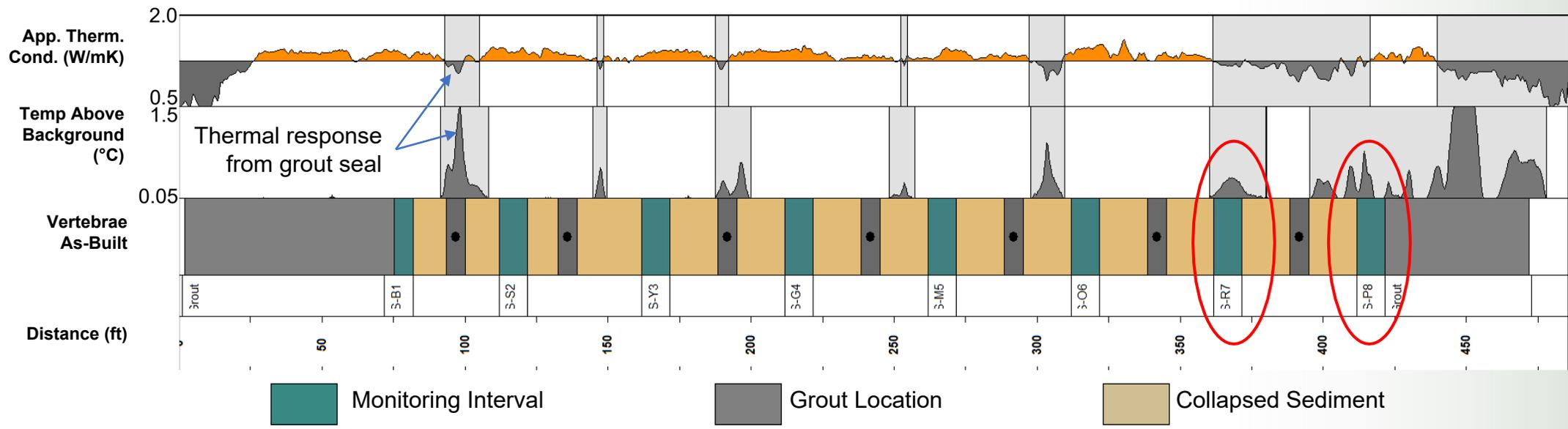
**Performance Objective:** Demonstrate integrity of grout seals to isolate individual screen segments
