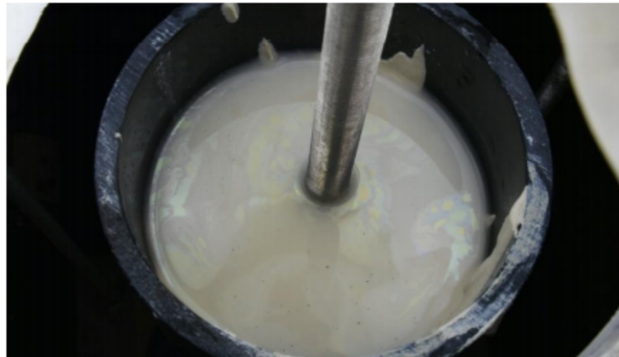
Oil: 400 \mu L OIL-2 Deposit: Consolidated Tool: Rod Drop with Manual Agitation Video/Photo No: 0684 (5)
